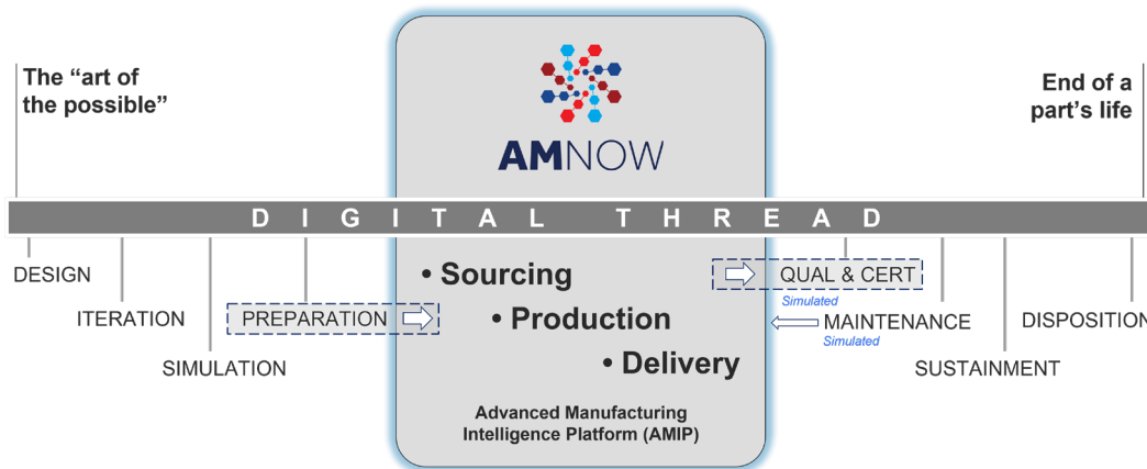
How AMNOW fits into the digital thread of the creation of a part
